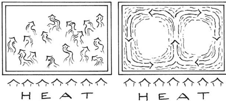
FIGURE 18. Demonstration of self-design in heating of water. Left: A steady pattern of heat conduction develops as heating proceeds. Right: Formation of Bénard convection cells at critical temperature differential.
